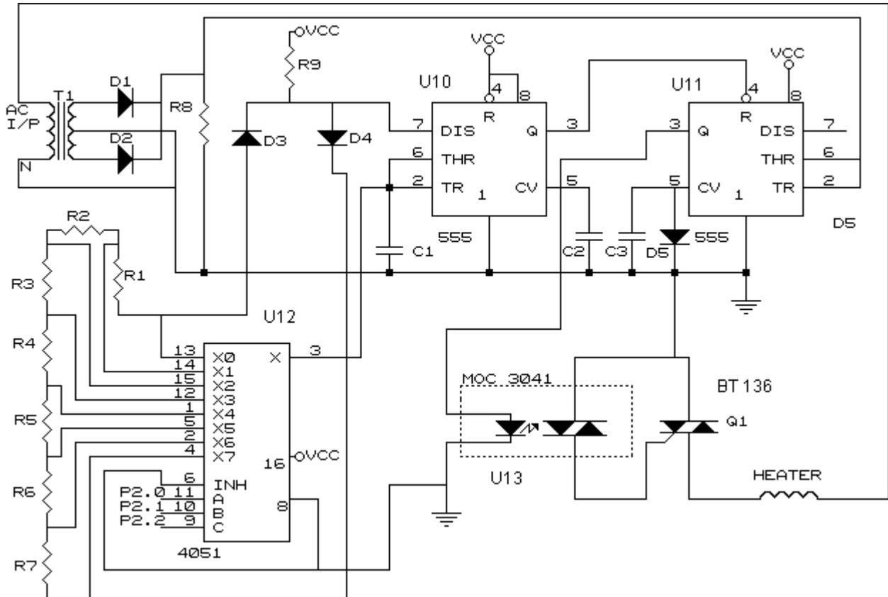
Fig. 4 Circuit Diagram for Solid State Power Controller
