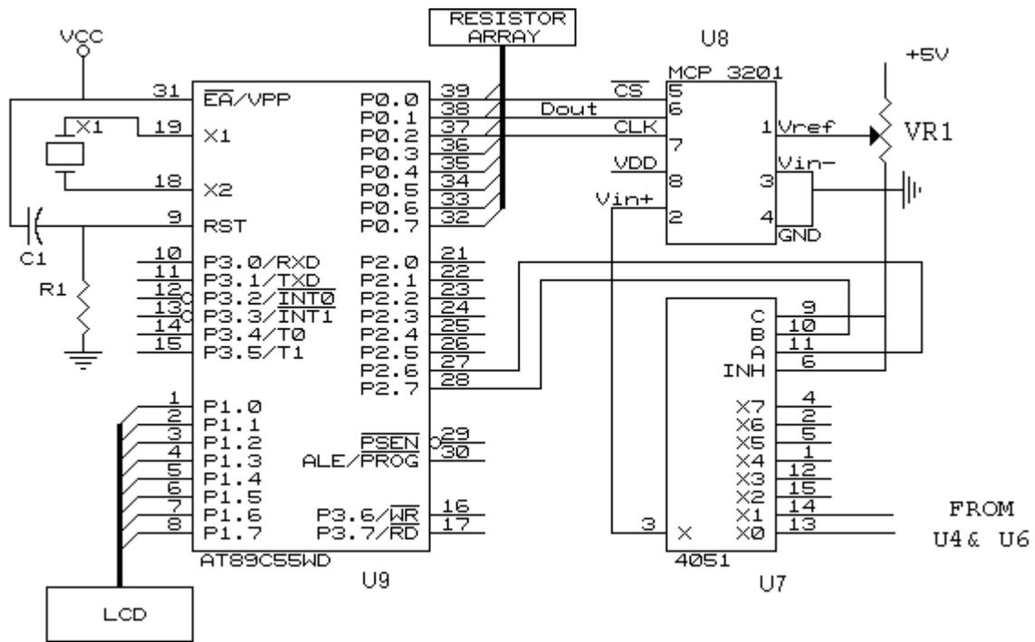
Fig. 3 Circuit Diagram of Microcontroller and 12-bit serial A/D Converter
