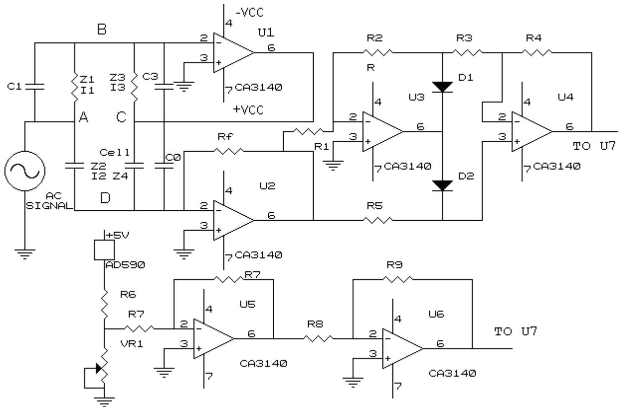
**Fig. 2** Modified AC Shering Bridge and Temperature Measurement Circuit
