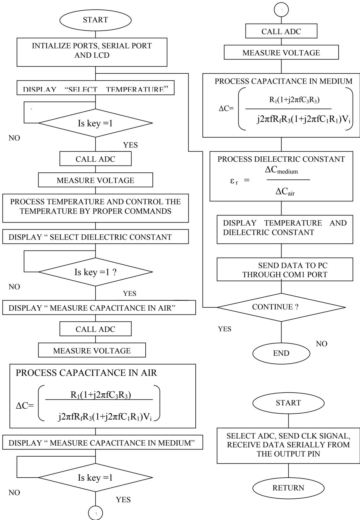
Fig.5 Flow Chart for Performing Dielectric Constant Measurement System
