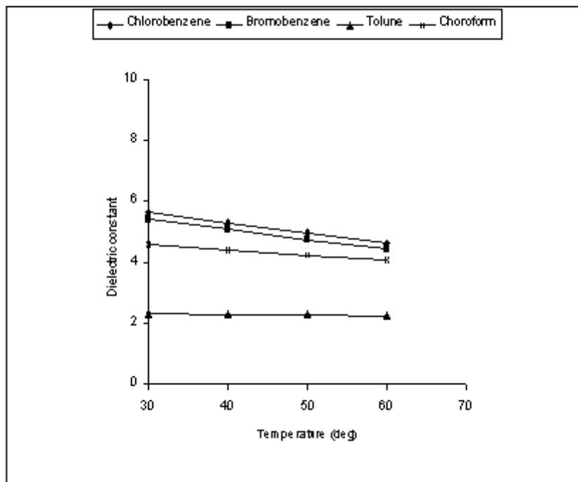
Fig. 7 The Dielectric Constant of Liquids at Various Temperatures
