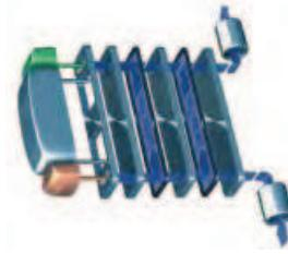
In an Alicat mass flow instrument, a discrete absolute pressure sensor and a temperature sensor are placed in the laminar region of the flow stream.
